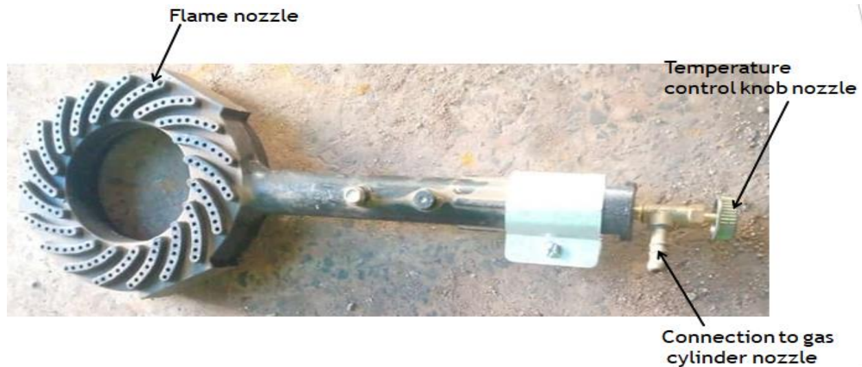
Figure 3 Gas burner and Temperature control knob
