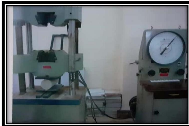
Figure 2.3 Setup of Indirect Tensile Test
