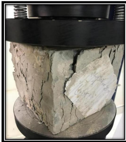
Figure 2.2 Failure pattern in concrete block after testing
