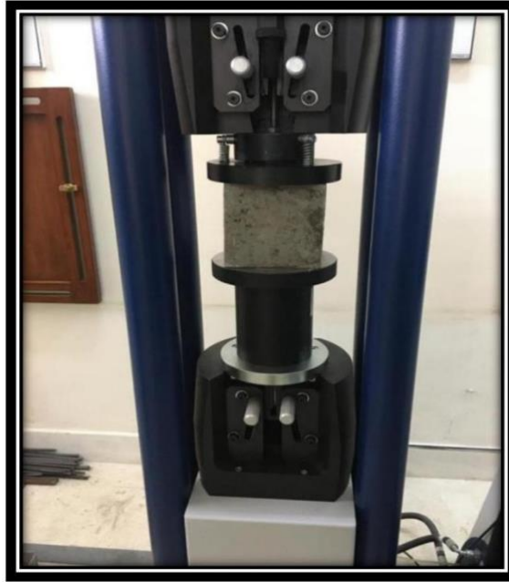
Figure 2.1 Placing of concrete block before testing
