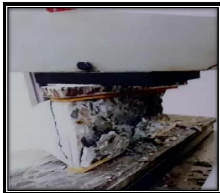
Figure 2.5 Failure pattern in concrete sample after Testing
