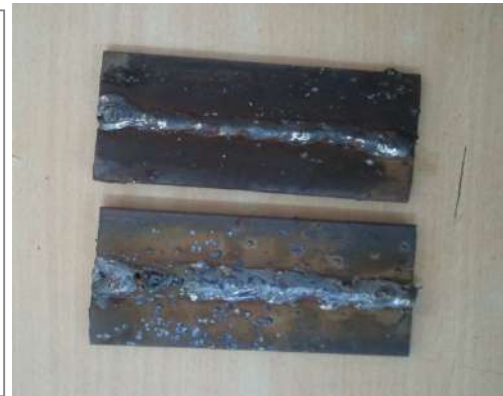
Fig 7. MIG welding of mild steel
