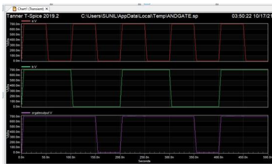
Fig 9. Simulation of OR gate without fault
