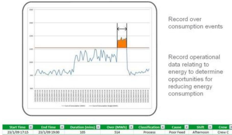
Figure 5 illustrates an “energy event” where over consumption of energy occurred. The MES captured context around this event and poor feed was attributed to the over consumption of energy.
