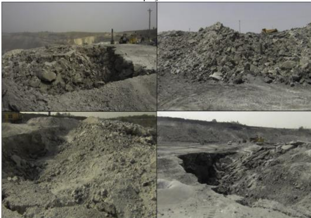
Fig. 4. View of the detonation sequence of shovel bench blast conducted at Kusmunda project.
